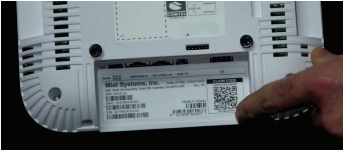
Figure 27: QR Code on an Access Point
